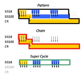
Figure 4: Pattern, chain, and super cycle, illustrated for the parallel operation of anti-proton production (orange) and RIB production (blue). The injector linacs as well as the HESR accumulating the anti-protons are omitted.
