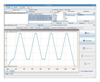
Figure 5: LSA application showing the main dipole field for a SIS18 super cycle in the FAIR injector mode.
