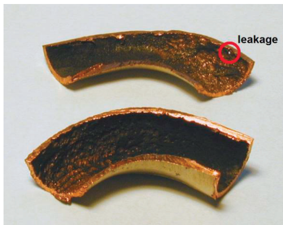
Fig.5: Water pipe with cavitation pits.
