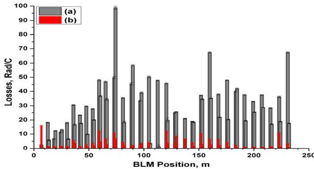
Figure 4: The BLM signals along the SCL normalized by charge of the beam transmitted to the SCL for (a)  $H^-$  ion and (b) proton beams. The Fig. is from [1].
