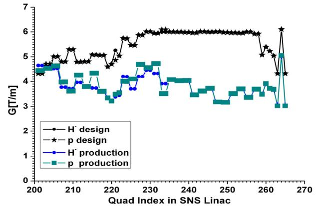
Figure 3: The SCL quadrupole gradients for different SCL optics.
