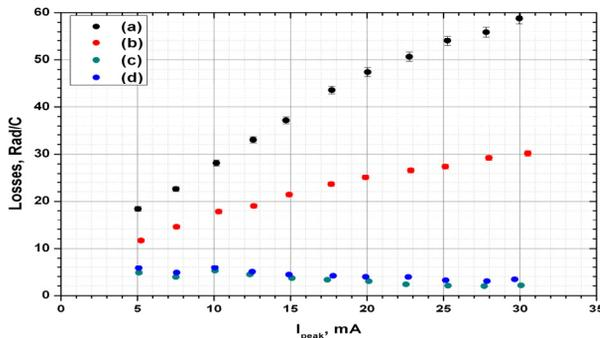
Figure 5: The normalized BLM signals vs. peak current for different beams and optics: (a) and (b)  $H^-$  beam for the design and production SCL optics respectively; (c) and (d) proton beam for the design and production SCL optics respectively.
