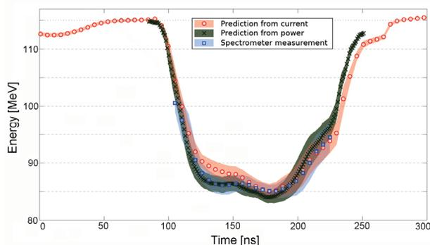
Figure 4: Comparison between the measured time-resolved beam energy profile and the predictions from beam current and power production measurements. Data were averaged over 48 consecutive pulses. The shaded areas indicate the standard deviation.
