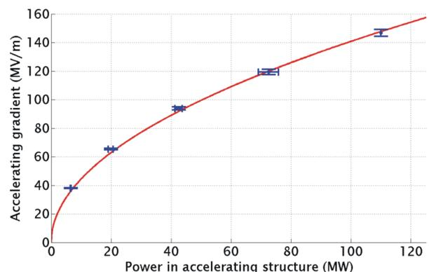
Figure 3: Measured accelerating gradient as function of the accelerating structure RF input power.
