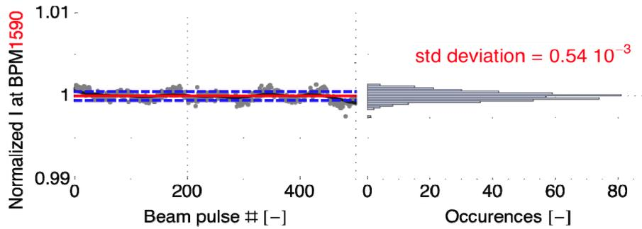
Figure 2: Pulse charge stability measurements in CTF3 (last linac BPM, with gun feedback on).
