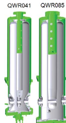
Figure 1: Two types of QWRs ( $\beta_{opt}=0.041$  left,  $\beta_{opt}=0.085$  right) used in FRIB linac, both operate at 80.5MHz.
