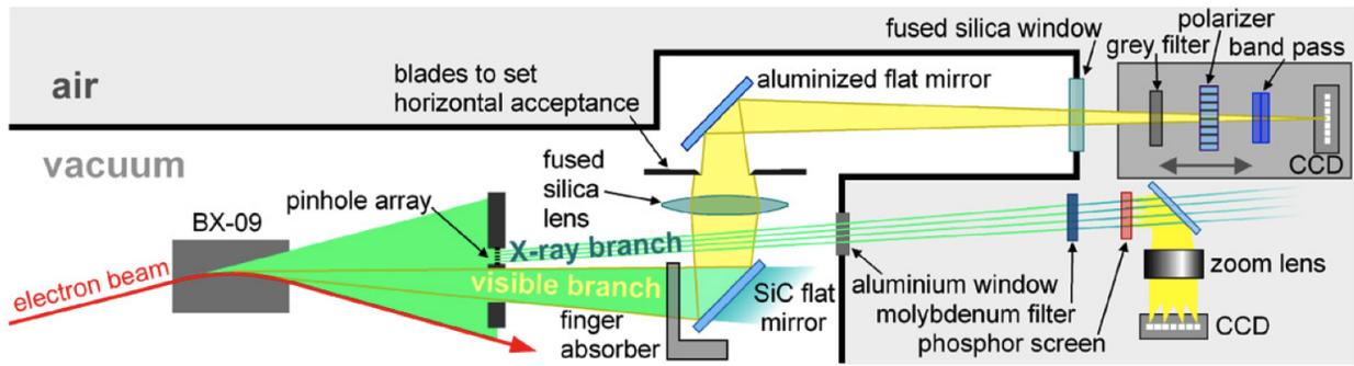
Figure 2: Schematics of the diagnostic beam line showing the vis-UV and the X-Ray branches.
