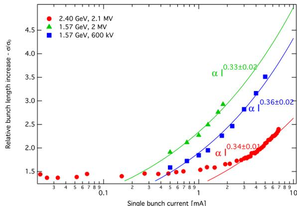
Figure 4: Measured bunch length as a function of single bunch current for 2.4 GeV ( $V_{rf}=2.1 \text{ MV}$ ) and 1.57 GeV ( $V_{rf}=600 \text{ kV}$  and  $2 \text{ MV}$ ). The lines are the fits to the turbulent regime and the exponents obtained in the fitting are shown beside each line.
