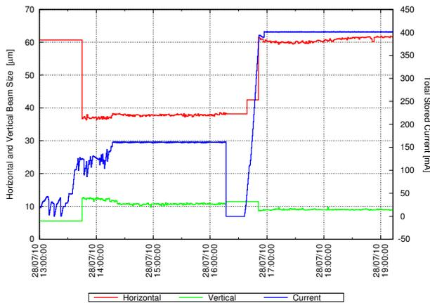
Figure 1: Machine shift showing the switch between 2.4 GeV mode to 1.57 GeV and back. Observe that the horizontal beam size drops from 60 μm to 38 μm, which corresponds to a change in emittance expected.
