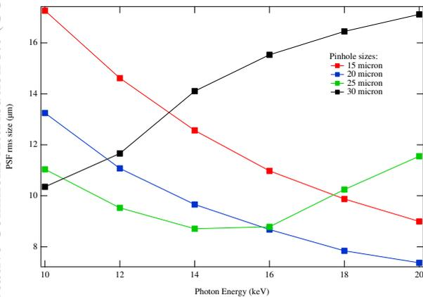
Figure 3: Calculated PSF for each pinhole size available in the SLS.
