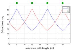
Figure 2: Betatron functions along two 54° FODO cells.
