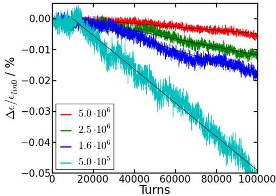
Figure 3: Decreasing emittances of beams with different numbers of macro particles. The data were smoothed to suppress noise.
