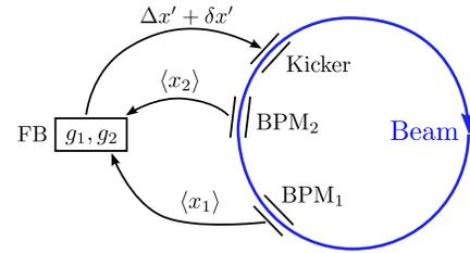
Figure 1: Feedback model implemented in BeamBeam3D.
