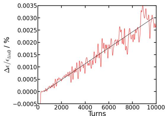
Figure 2: Emittance growth in a self-consistent simulation. The data were smoothed to suppress noise.
