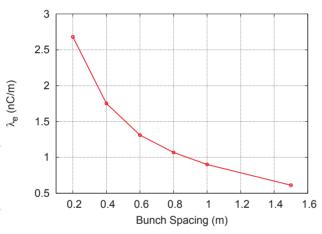
Figure 3: Variation of saturated line density with bunch spacing. Simulations have been run for 3350 consecutive bunches.
