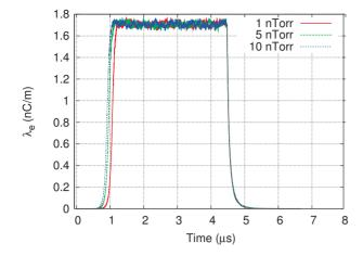
Figure 6: Evolution of electron cloud density with time for 3350 consecutive bunches at residual gas pressure 1, 5 and 10 nTorr.
