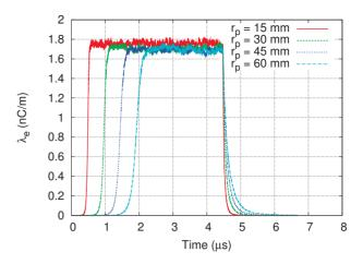
Figure 4: Time evolution of electron cloud for beam pipe with different radii. Simulations are run for 3350 consecutive bunches.
