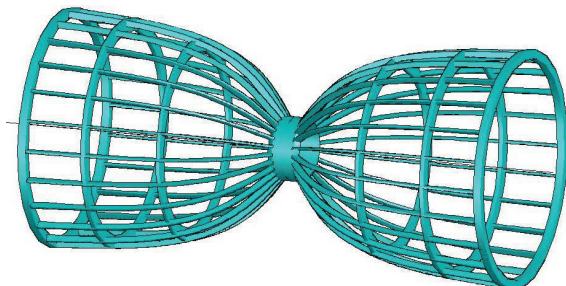
Figure 10: A Conceptual design of the lens. Double paraboloid type. Conductors jointed by welding. Cooling tubes are running in a body of each conductor.
