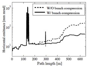
Figure 7: Beam tracking simulation with and without bunch compression in the J-ARC.
