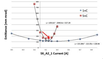
Figure 3: Initial offset scan to compensate transverse wakefiels.
