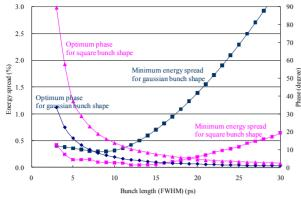
Figure 5: Minimum energy spread and optimum phase.
