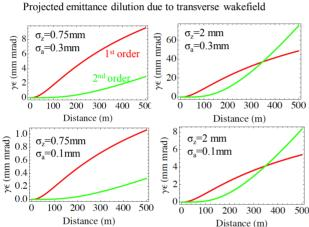
Figure 6: Consideration of bunch compression using J-ARC.
