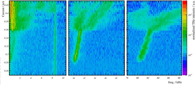
Figure 1: Instability spectrum of low frequency bursting is shown on the left diagram. Bursting occurs at currents > 0.28 mA and changes mode at 0.36 mA. The main instability can be found at about 400-600 Hz and drifts with the current. Its harmonics are also clearly observable. The  $1f_s$  frequency line can be seen at 8.5 kHz. The middle and left figure show typical bursting patterns with onset at the same thresholds.
