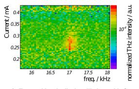
Figure 3: Expected longitudinal oscillations with  $f_s$  cause  $2f_s$  fluctuations of CSR. It is remarkable that this line appears only around the onset of bursting at 0.24 - 0.30 mA
