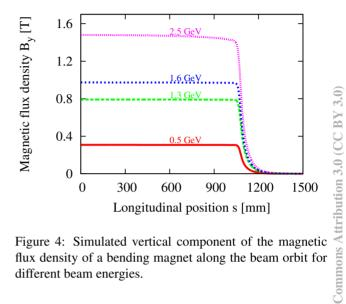
Figure 4: Simulated vertical component of the magnetic flux density of a bending magnet along the beam orbit for different beam energies.
