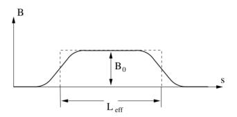
Figure 1: (Schematic diagram).  $B_0$  is a maximum magnetic flux density.  $L_{\rm eff}$  is an effective bending magnet length.
