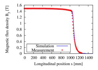
Figure 3: Simulated and measured vertical component of the magnetic flux density of a bending magnet along the beam orbit.
