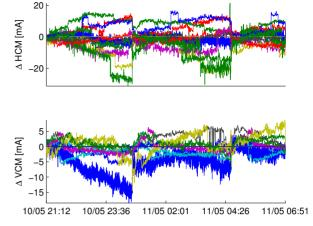
Figure 4: Change in the corrector strength for the first corrector in each sector. The upper figure shows the horizontal correctors and the lower the vertical ones. 20 mA of current correspond to a 2  $\mu$ rad kick. The large changed observed for example in the blue line in the vertical correspond to the injection.
