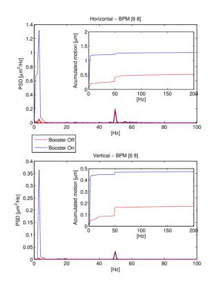
Figure 7: Power spectral density and accumulated motion for the 10 kHz sample data of the orbit, with the booster on and off. The large component at 3.125 Hz is the effect of the booster, but the accumulated motion is under the  $\mu$ m in the vertical and barely over it in the horizontal.
