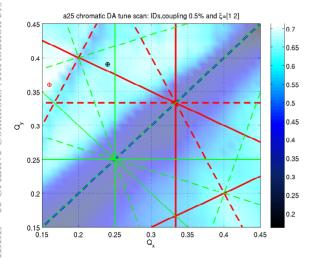
Figure 1: Chromatic dynamical aperture simulations as a function of the working point. The starting working point is repesented by a black cross while the new working point is in red.
