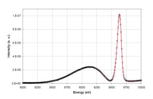
Figure 7: Comparison of the theoretical spectrum to the measured one for one of the in-vacuums undulators. All the nominal settings agree well, with just the energy fitted to 2.998 GeV.
