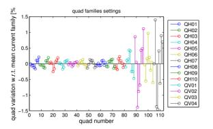
Figure 3: Quadrupole change applied to symmetrize the ALBA storage ring optics with LOCO.
