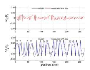
Figure 5: The horizontal (top) and vertical (bottom) beta beating intruduced by the supeconducting wiggler: the model values are compared with the measured ones.
