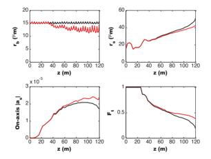
Figure 1: On-axis  $|a_s|$ ,  $r_s$  and  $F_t$  with constant (black lines) and varied (red lines)  $r_b$ , obtained by GENESIS single-frequency simulation. The oscillation in  $r_b$  is due to imperfect matching of the transverse optics.
