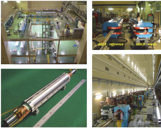
Figure 4: (1) upper left; experimental decks for vacuum works at the KEKB Oho laboratory, (2) upper right; the magnetic measurement bench for new dipole magnets for the LER, (3) lower left; the QC1P R&D magnet, and (4) lower right; six ARES cavities relocated from the HER to the LER beam line in the D5 straight section.
