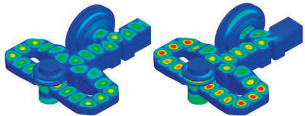
Figure 2: Electric field plots for the reflector in ON (left) and in OFF (right) positions.
