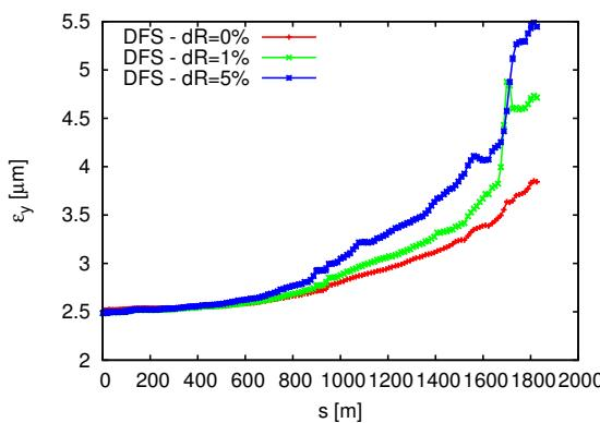
Figure 3: Emittance growth after dispersion-free steering with imperfect model, compared to the case with perfect mode. The results are the average of 1000 random seeds.
