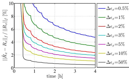
Figure 1: Convergence of the system identification algorithm. A relative error of 1% is considered sufficient to perform BBA. The result is the average of 100 random seeds.
