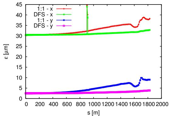
Figure 2: Emittance growth with static imperfections, after beam-based alignment. The result is the average of 100 random seeds.
