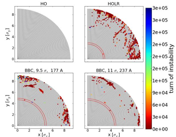
Figure 5: Particle stability for the nominal LHC optics and a crossing angle corresponding to  $9.5\sigma$  separation considering the same four cases as in Fig. 4.
