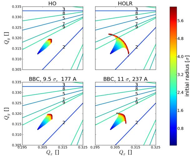
Figure 4: Tune footprint for the nominal LHC optics and crossing angle corresponding to a  $9.5\sigma$  separation, with HO only (top left) HOLR (top right), BBC wire at  $9.5\sigma$  (bottom left) and BBC wire at  $11\sigma$  (bottom right).
