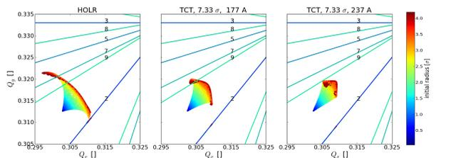
Figure 8: Tune footprints for the modified LHC optics and a reduced crossing angle corresponding to  $6.3\sigma$  separation.
