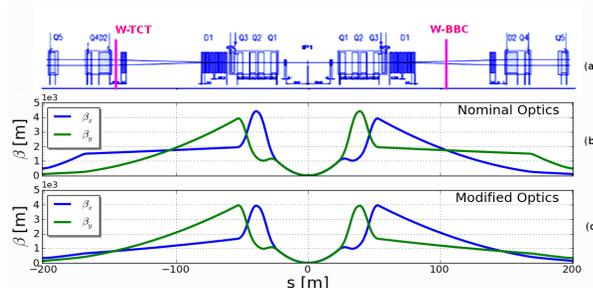
Figure 1: Wire locations (top), and  $\beta$  functions for the nominal (center) and the modified optics (bottom).
