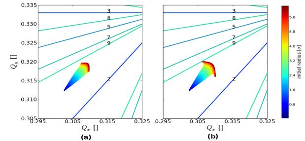
Figure 10: Tune footprints for the nominal optics with a BBC wire, for a pencil (left) and a square-rod wire (right).
