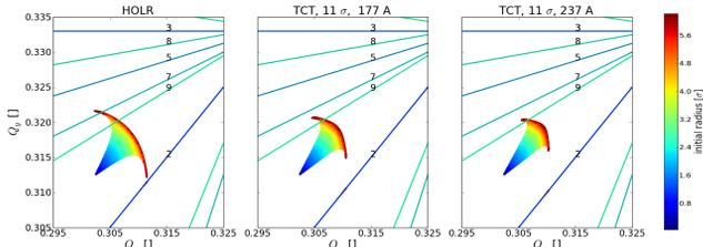
Figure 6: Tune footprints for the modified LHC optics and a crossing angle corresponding to  $9.5\sigma$  separation.
