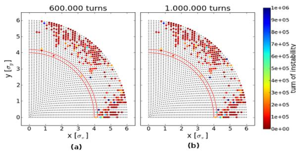
Figure 3: Particle stability for HOLR with a reduced crossing angle corresponding to a LR separation of  $6.3\sigma$ , when tracking over  $6 \times 10^5$  (left) or  $10^6$  turns (right).
