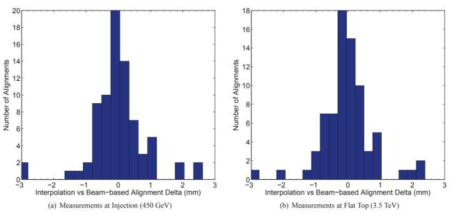
Figure 2: Delta between the BPM-interpolated and the beam-based centers at the LHC collimators in 2011.
