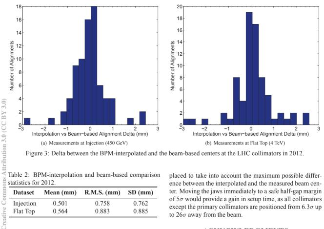
Figure 3: Delta between the BPM-interpolated and the beam-based centers at the LHC collimators in 2012.
