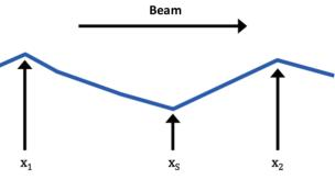
Figure 1: Example of the beam orbit through points 1, S and 2 (from [3]). With BPMs located at point 1 and 2, the objective of the interpolation is to find the orbit at point S.
