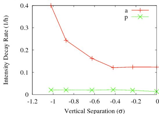
Figure 1: Beam intensity decay rate as a function of vertical beam-beam separation at one collision point. ‘a’- antiproton data, ‘p’- proton data.
