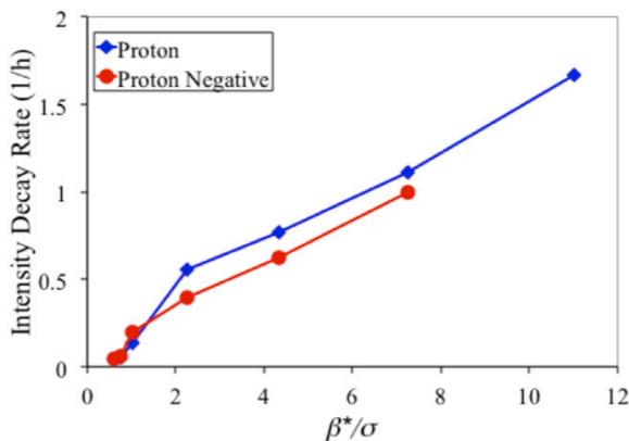
Figure 3: Proton beam intensity decay rate as a function of  $\beta^*$  to bunch length ratio.
