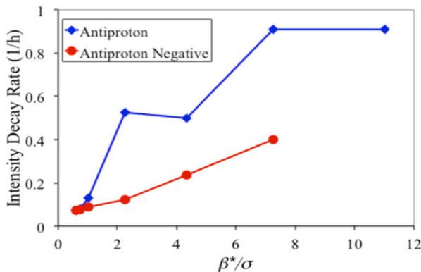
Figure 4: Antiproton beam intensity decay rate as a function of  $\beta^*$  to bunch length ratio.
