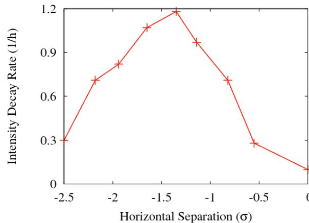
Figure 2: Antiproton beam intensity decay rate as a function of transverse beam-beam separation at one collision point.
