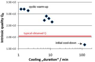
Figure 1: Dependence of obtained  $Q_0$  on cool-down speed. Measurements were taken at 1.8K and  $E_{acc}=4MV/m$ .
