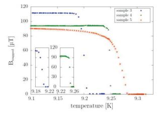
Figure 4: Flux release as a function of sample preparation history. Polycrystalline, BCP treated and post annealed at 800°C (blue squares); single crystal, BCP treated (green triangles); single crystal, BCP treated and post annealed at 800°C (red crosses). The time step between two neighbouring points is 1 sec. Note that slightly different field levels were applied and the thermo sensors had slightly different offsets.
