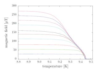
Figure 5: Flux release of different levels of trapped magnetic field in a single crystal Niobium sample (BCP + 1200°C) upon heating in zero external field.
