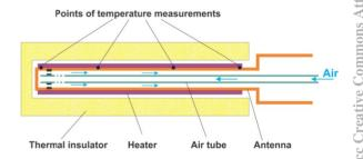
Figure 4: Scheme of measurements of antenna air cooling effectiveness.
