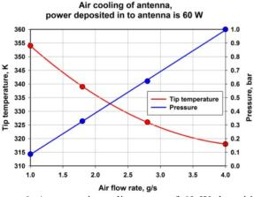
Figure 6: Antenna air cooling, case of 60 W deposition into antenna (650MHz, 120kW, TW). ~2.5g/s flow rate and ~0.5 bar pressure provide acceptable temperature of antenna tip. Thermal radiation at this point ~0.1W.
