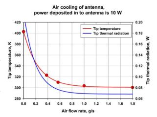
Figure 5: Antenna air cooling, case of 10 W deposition into antenna (325MHz, 30kW, TW). ~0.3 g/s flow rate provides acceptable temperature of antenna tip. Thermal radiation at this point ~0.1W.
