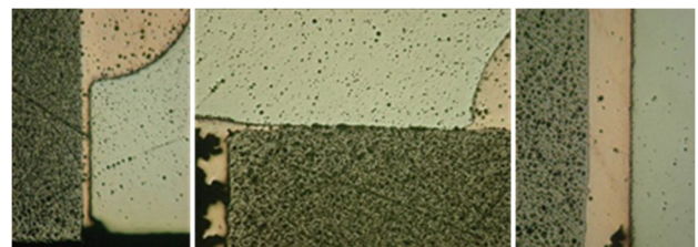
Figure 7 : Micrographs of the large trial pieces showing uniform copper filler material in each of the three areas of the joint.
