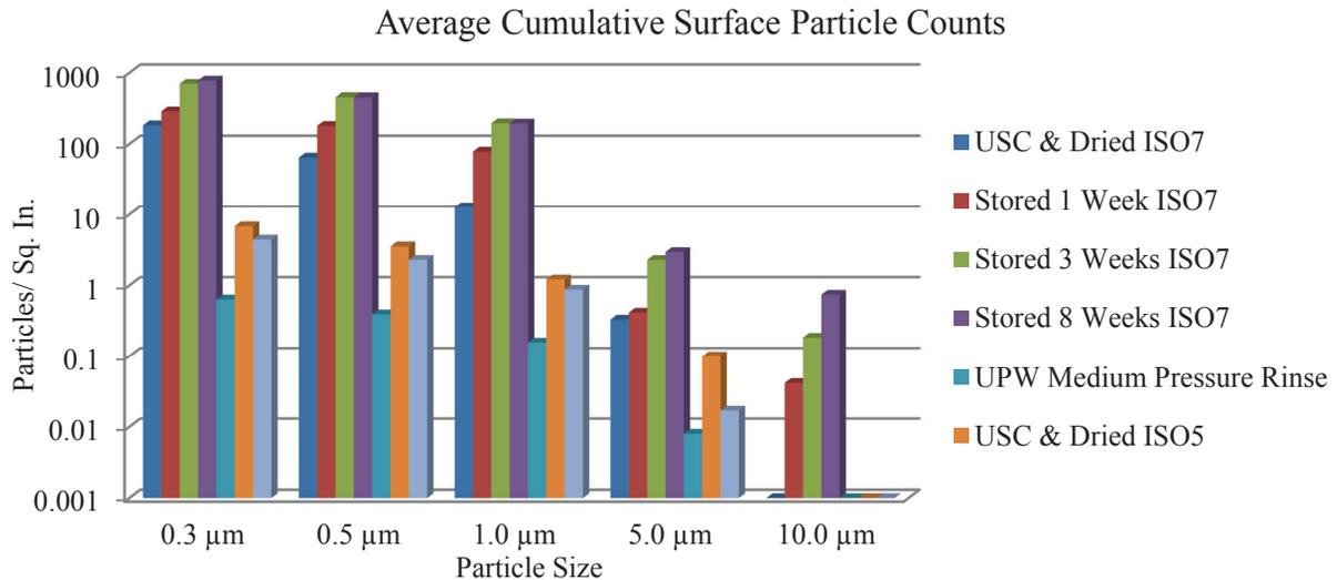
Figure 2: Cleaning and storage techniques comparison for 2.75" conflat flanges.
