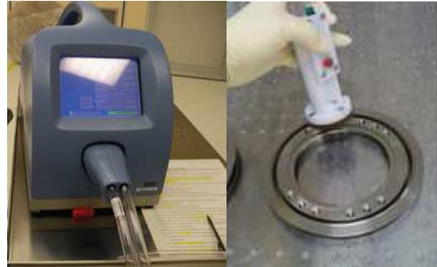
Figure 1: QIII+ surface particle counter and 2" probe scanning titanium blind tapped holes flange.
