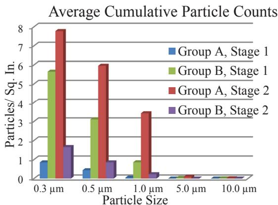
Figure 4: Surface particle count data of two stages of different procedures on tuning plates.
