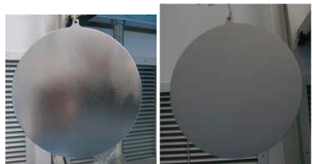
Figure 3: Nb Sample plate before (left) and after (right) Nb 3 Sn coating
