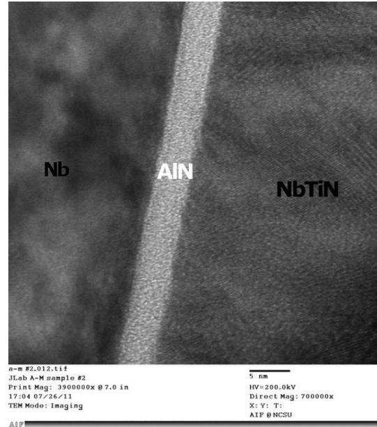
Figure 2: TEM image of a FIB cut NbTiN/AlN/Nb/Cu structure.
