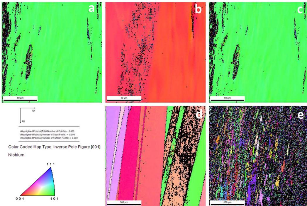
Figure 1: EBSD maps of Nb films grown on Cu (a, b, c) single crystal (100), (110), (111), polycrystalline (c) large grains and (d) fine grains simultaneously [10].
