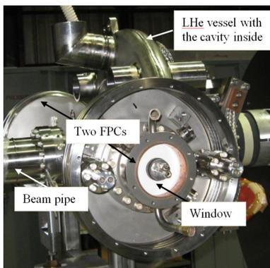
Figure 1: BNL SRF gun with two opposing FPCs attached.
