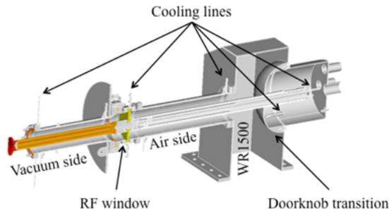
Figure 2: Design of 500-kW fundamental power coupler.
