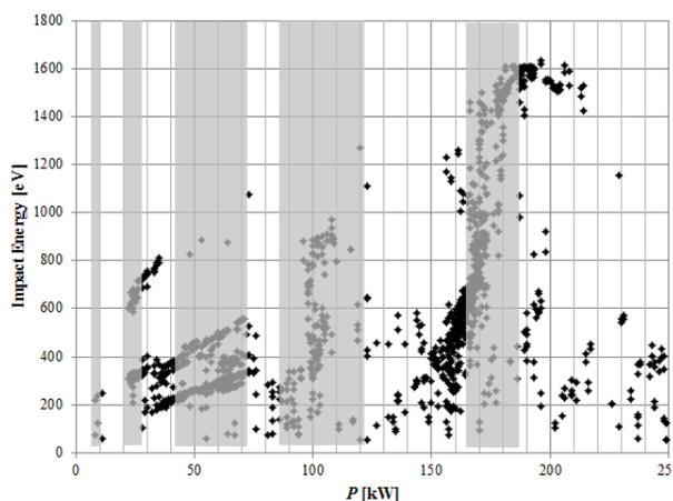
Figure 8: Comparison of multipacting zones from FPC conditioning test (grey-shaded areas) and simulation results at 703.9 MHz with 0 degree (black dots).
