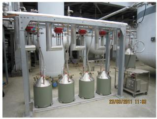
Figure 3: Adsorbers of the purifier system.
