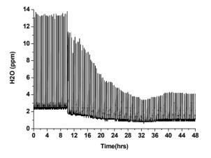
Figure 5: Moisture reading of the analyzer during cryogenic system operation.
