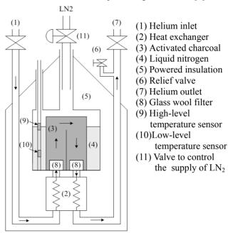
Figure 2: Cryogenic adsorber.
