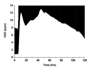
Figure 6: Moisture reading of the analyzer during cryogenic plant and superconducting devices warm up.
