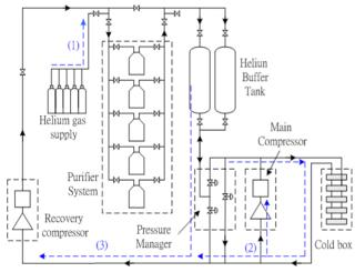
Figure 4: Configuration of the purifier system.
