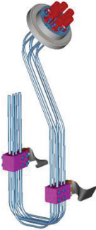
Figure 5: Conduction cooled lead assembly.
