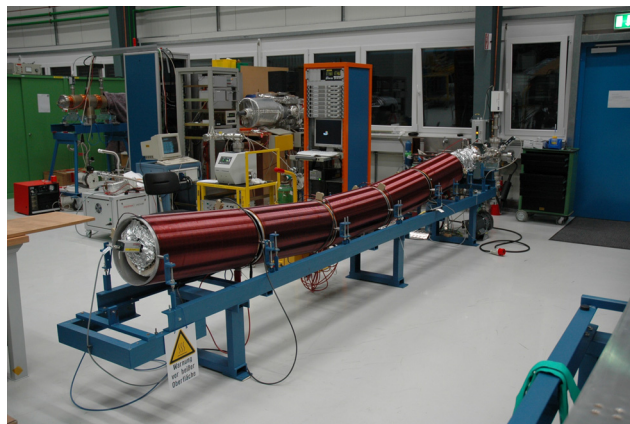
Figure 1: Magnetron sputtering facility designed and commissioned at GSI to perform the NEG coating of the dipole magnet chambers of the SIS 18.
