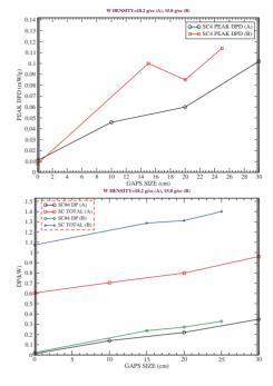
Figure 5: Peak deposited power density in coil SC 4 (top), and total deposited power in SC 4 and in all SC coils (bottom), *vs.* axial gap in the shielding. Both plots show results for W densities of 15.8 and 18.2 g/cm<sup>3</sup>.
