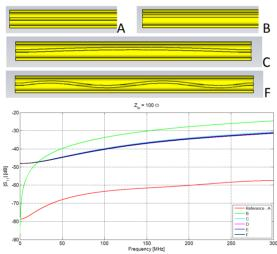
Figure 8: Effect of offset and undulations for the different structures. C, D, E, F have 0.5, 1, 1.5 and 2 - oscillations, respectively, as shown just for C and F.
