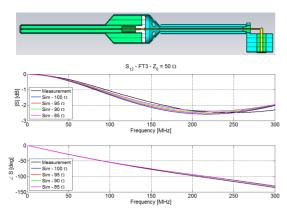
Figure 7: CST Microwave Studio simulation geometry and results of measurements fitting.
