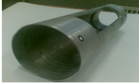
Figure 7: Aluminium buncher Prototype for measurement precision of manufacturing by CMM.
