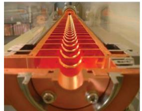
Figure 4: A cut-view of 2-m accelerator section.
