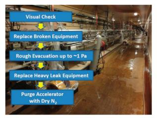
Figure 5: The linac vacuum purge with dry nitrogen.
