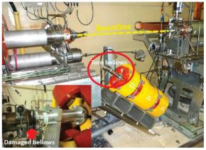
Figure 1: The linac damage in accelerator tunnel.
