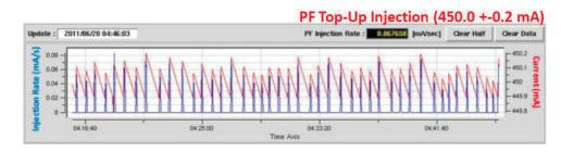
Figure 6: Accumulation current and rate of the PF storage ring.
