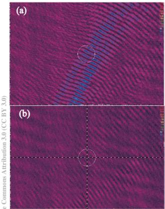
Figure 3: Typical background images of the laser beam (a) without any baffles and (b) with five baffles obtained at the focal region without any FZPs. In this measurement, the gain of the CCD camera was set to be 16 dB.
