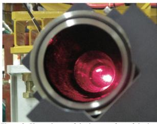
Figure 2: Photo-picture of the inner surface of the laser pipe viewed upstream from the location at the distance of L = 13.385 m.
