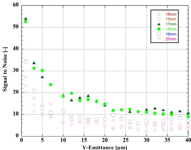
Figure 3: S/N of structure transmission from simulations.
