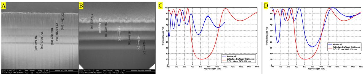
Figure 1: SEM micrographs of DBR cross-sections for the MAP structure upper slab: (a) before calibration of the deposition machine; (b) after. Comparison of transmittance measurements on structures (blue) and simulation using ideal dimensions (red): (c) for the structure labeled A; (d) for the structure labeled B.
