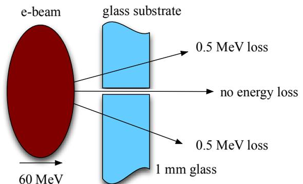
Figure 2: Transmission model of beam through structure.
