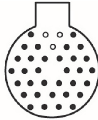
Figure 2: The schematic of the arrangement of the rods in the coupler cells. White circles correspond to the removed rods.
