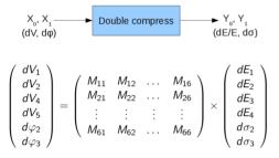
Figure 4: Response matrix transforming variations of the beam parameters to RF voltage and phase corrections.
