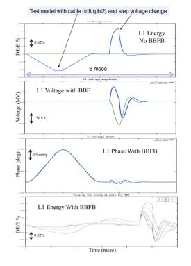
Figure 5: Initial results from the model for a single linac/bunch compressor module. a) Energy drift from RF cable drift (phi2) and a step voltage change. b) Effect of beam-based FB on voltage set point. c) effect of beam-based FB on phase set point. d) Energy drift with RF and beam-based FB at different gains.
