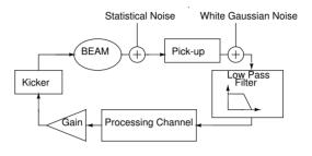
Figure 1: Complete feedback loop.
