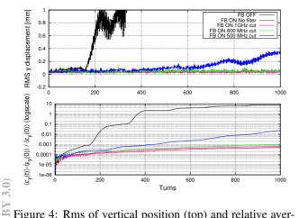
Figure 4: Rms of vertical position (top) and relative average vertical emittance growth (bottom) of the beam in the case of FB OFF (black) and FB ON with no filter (red), with filter cut off at 1GHz (magenta), 800 MHz (green) and 500 MHz (blue).
