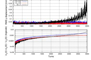
Figure 6: Rms of vertical position (top) and relative average vertical emittance growth (bottom) of the beam in the case of gain G = 0.2 (blue), G = 0.5 (red) and G = 1 (black).
