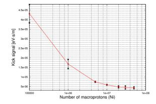
Figure 2: Minimum kicker signal required to stabilize the beam (i.e. for the vertical emittance to grow less than 0.1% over 1000 turns) as a function of  $N_i$ . The black vertical bars correspond to the error intervals, the amplitude of each interval is related to the number of simulations performed for each  $N_i$  value.
