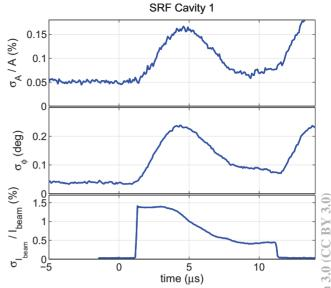
Figure 9: Noise in amplitude and phase of the SRF cavity 1 field and in the beam current.
