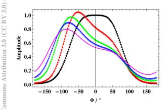
Figure 2: Beam distribution deformation and phase shift by PWD using  $Z_{SC||}$  in Equation 2. The quality factor Q = 0.1. Black points: no PWD ( $\Sigma = \frac{1}{(\frac{V_{BE}}{V_{SC}}-1)} = 0.0$  as defined in [1], no beam), red triangles:  $N_b = 4 \cdot 10^{10} (\hat{=}\Sigma = 0.1)$ , green squares:  $N_b = 9 \cdot 10^{10} (\hat{=}\Sigma = 0.3)$ , blue stars:  $N_b = 13 \cdot 10^{10} (\hat{=}\Sigma = 0.5)$  and pink line:  $N_b = 20 \cdot 10^{10} (\hat{=}\Sigma = 1.0)$ .
