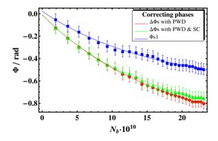
Figure 6: Phase advance over number of ions  $N_b$  for beam distribution deformation- and phase shift correction with measured impedance table.
