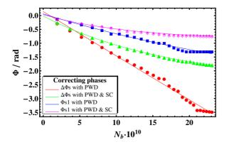
Figure 5: Phase advance over number of ions  $N_b$  for beam distribution deformation- and phase shift correction with Q = 0.1 by using impedance function Equation 2.
