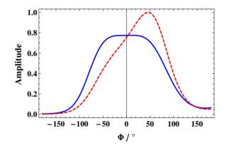
Figure 4: Correction of phase shift by  $\Phi_{S1}$  using Equation 2 (bottom). Red dashed line: bunch form distribution without PWD, blue line: bunch form distribution with PWD after phase shift and deformation correction.
