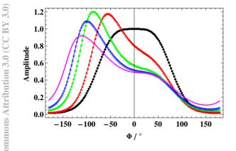
Figure 1: Beam distribution deformation and phase shift by PWD using  $Z_{Sh||}$  in Equation 2. The quality factor Q = 0.1. Black points: no PWD ( $N_b = 0.0$ ), red triangles:  $N_b = 4 \cdot 10^{10}$ , green squares:  $N_b = 9 \cdot 10^{10}$ , blue stars:  $N_b = 13 \cdot 10^{10}$  and pink line:  $N_b = 20 \cdot 10^{10}$ .
