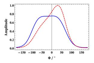
Figure 3: Correction of beam distribution deformation by  $\Delta \Phi_S$  using Equation 2 (top). Red dashed line: bunch form distribution without PWD impedance, blue line: bunch form distribution with PWD after deformation correction.
