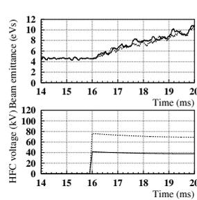
Figure 6: The variation of the longitudinal beam emittance and the high frequency voltage (16 ms start).
