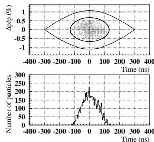
Figure 5: The beam emittance and the bunch shape (18 ms start,  $h_b/h_0 = 30$ ).
