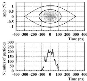
Figure 2: The beam emittance and the bunch shape (16 ms start,  $h_b/h_0 = 20$ ).
