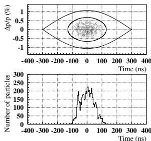
Figure 4: The beam emittance and the bunch shape (18 ms start,  $h_b/h_0 = 20$ ).
