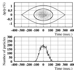
Figure 9: The beam emittance and the bunch shape (16 ms start,  $h_b/h_0 = 30$ ).
