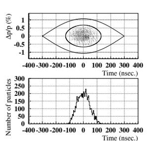
Figure 11: The beam emittance and the bunch shape (18 ms start,  $h_b/h_0 = 30$ ).
