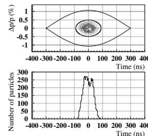
Figure 1: The longitudinal beam emittance and the bunch shape at the RCS extraction. No blow-up is applied.
