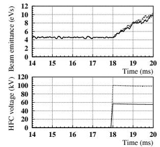
Figure 7: The variation of the longitudinal beam emittance and the high frequency voltage (18 ms start).
