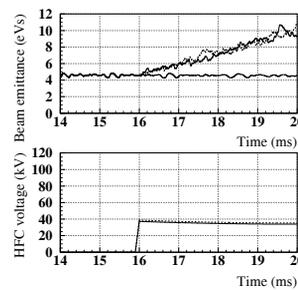
Figure 12: The variation of the longitudinal beam emittance and the high frequency voltage (16 ms start).
