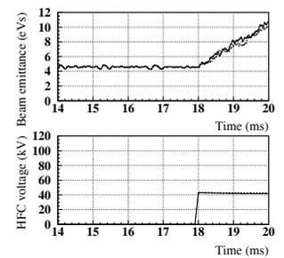
Figure 13: The variation of the longitudinal beam emittance and the high frequency voltage (18 ms start).
