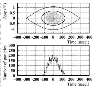
Figure 8: The beam emittance and the bunch shape (16 ms start,  $h_b/h_0 = 20$ ).
