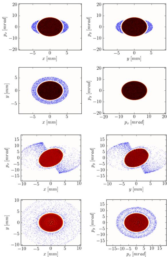
Figure 2: After 500 passes in the linear lattice, the initial pre-halo (top) has begun large radius oscillations (bottom).
