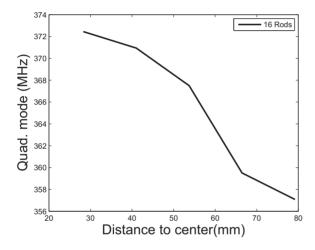
Figure 7: Variation of the quadrupole resonance frequency for different slug tuner penetration.
