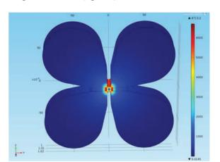
Figure 1: Abs. E field (V/m) for a Quadrupole mode representation in a 20mm (Z axis) Cold-Model section. Frequency = 352.2 MHz.
