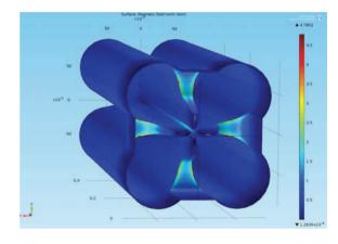
Figure 5: Abs. Magnetic field (A/m) on the RFQ ends for the quadrupole mode.
