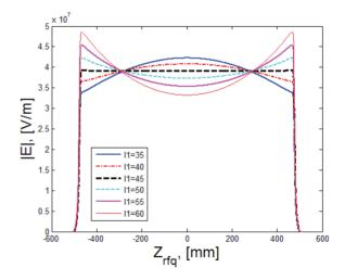
Figure 6: Variation in field flatness along a non modulated 1m RFQ regarding the penetration of the lobe inside the cavity  $(l_1)$ .
