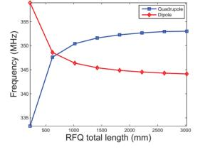
Figure 3: Variation of the RFQ resonant modes with total length.
