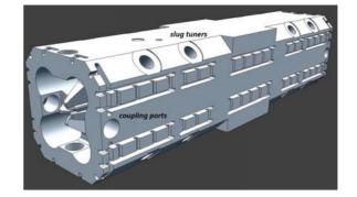
Figure 8: Layout of the ESS-Bilbao RFQ Cold-Model. Where L=1067.4 mm is the total length, h=w=260 mm are height and width,  $\phi_{tuner}=35$  mm is the tuner diameter and  $\phi_{coupler}=21.27$  mm is the diameter of the input power ports.
