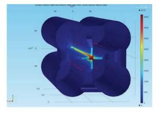
Figure 4: Abs. Electric field (V/m) on the RFQ ends for the quadrupole mode.
