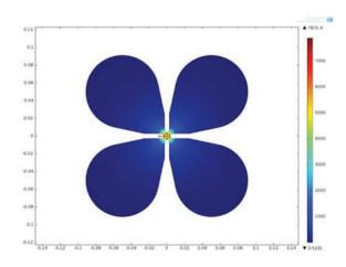
Figure 2: Abs. E field (V/m) for a 2D Dipole mode representation (XY plane at Z=0.5m). Frequency = 346 MHz.
