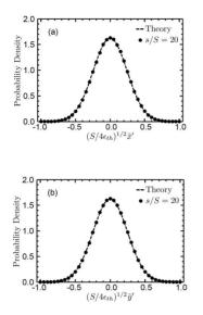
Figure 3: Plots of (a) probability density distributions  $\rho(\tilde{x}')$  versus  $(S/4\varepsilon_{th})^{1/2}\tilde{x}'$  and (b) probability density distributions  $\rho(\tilde{y}')$  versus  $(S/4\varepsilon_{th})^{1/2}\tilde{y}'$  at s/S = 20. The dotted curves are from the PFB2D simulation, whereas the dashed curves are from the theoretical predictions [1-3].
