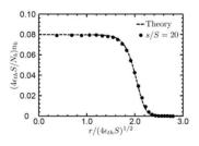
Figure 4: Plot of the normalized beam density  $(4\varepsilon_{th}S/N_b)n_b$  versus the normalized radius  $(S/4\varepsilon_{th})^{1/2}r$  at s/S = 20.
