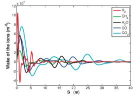
Figure 2. Wake field due to the ions along the whole ring with KCS beam. The total vacuum pressure is 0.5 nTorr with partial gas pressures shown in Table1.
