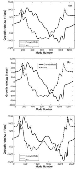
Figure 3. Calculated growth rate and frequency shift due to ions for different beams (a) KCS; (b) DRFS; (c) FF upgrade.
