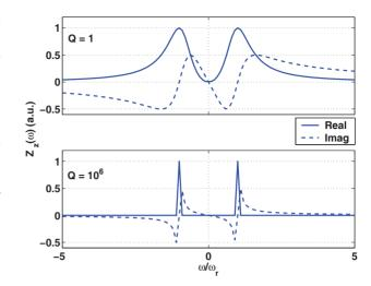
Figure 2: Illustration of longitudinal impedance for broadband (Q = 1) and narrow band ( $Q = 10^6$ ) RF structure.
