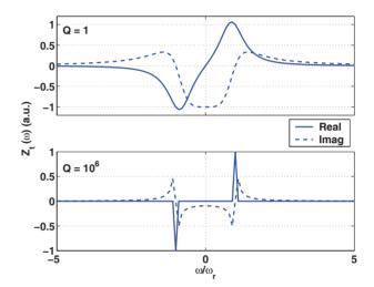
Figure 3: Illustration of transverse impedance for broadband (Q = 1) and narrow band ( $Q = 10^6$ ) RF structure.
