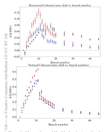
Figure 1: Measured tune shifts (black points) vs. bunch number, for a train of 10 0.75 mA/bunch 5.3 GeV positron bunches with 14 ns spacing, followed by witness bunches. Red points are computed (using POSINST) based on direct radiation and an ad-hoc assumption about the scattered photons. Blue points are computed using results from SYNRAD3D as input to POSINST.
