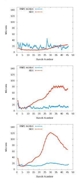
Figure 5: Bunch-by-bunch beam size and rms motion at 14 ns spacing and 2.1 GeV. Top: bunch current 0.5 mA/bunch (128 turns). Center: bunch current 1 mA/bunch (4096 turns). Bottom: Bunch current 1.3 mA/bunch (4096 turns).
