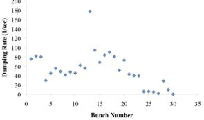
Figure 4: Vertical damping rate vs. the bunch number of a 30-bunch-long train of positrons at 2.1 GeV. Chromaticity: (H, V) =(0.58, 2.13) and the vertical feedback setting is 20% of full scale. Top: m=0 mode. Bunch current = 0.72 mA; estimated single bunch damping rate of 200 s<sup>-1</sup>. Bottom: m=-1 head-tail mode. Bunch current = 0.75 mA; estimated single bunch damping rate of  $110 \, \mathrm{s}^{-1}$ .
