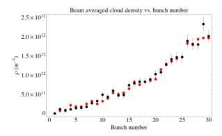
Figure 3: Data set 166: Average initial (i.e., before the "pinch") electron cloud density vs. bunch number, comparison between estimate from measured tune shifts (red), and simulation (black) from POSINST.
