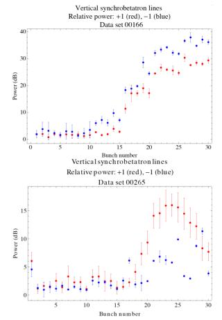
Figure 2: Vertical head tail lines, peak power vs. bunch number. Top: Data set 166: 2.1 GeV. Chromaticity: (H,V) = (1.33, 1.16). Bunch current = 0.74 mA. Bottom: Data set 265: 4 GeV. Chromaticity: (H,V) = (1.3, 1.4). Bunch current = 1.1 mA.
